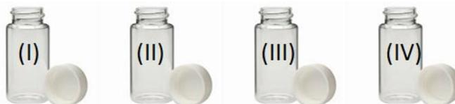
3. In all four vials, add 2 ml of solution (A). Use the plastic syringe to measure the volume and transfer the solution. For step 3,4,5 and 8, a separate syringe should be used to transfer each solution. Each group will need four syringes. It will be convenient to label each syringe A,B, C and E.
