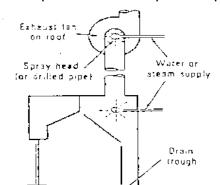
Perchloric acid fume hoods: Anyone working with perchloric acid must use a perchloric acid fume hood. These special fume hoods are equipped with a water spray system to wash down the
