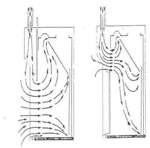
Diagram of an Auxiliary Air Fume Hood (Left – with sash open; Right – with sash lowered)
