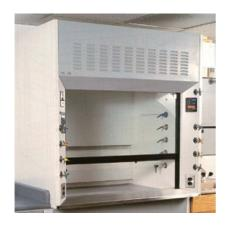
Similarly, a supply air vent located directly above a fume hood can also cause turbulence in the hood.
