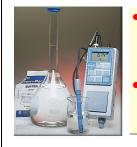
The solid acid and conjugate base in the packet are mixed with water to give the specified pH.
