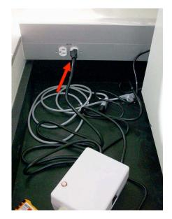
2. Plug in the cable of the microwave reactor into one of the two plugs at the front of the power converter.
