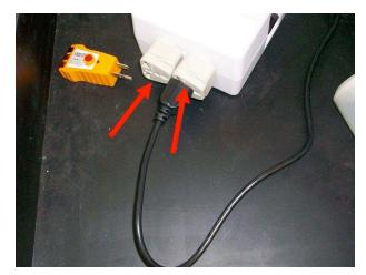
3. Switch on the power supply on the power converter (left) and finally switch on the microwave reactor (right).
