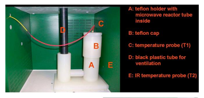
1. Place the reactor tube in the Teflon holder.
