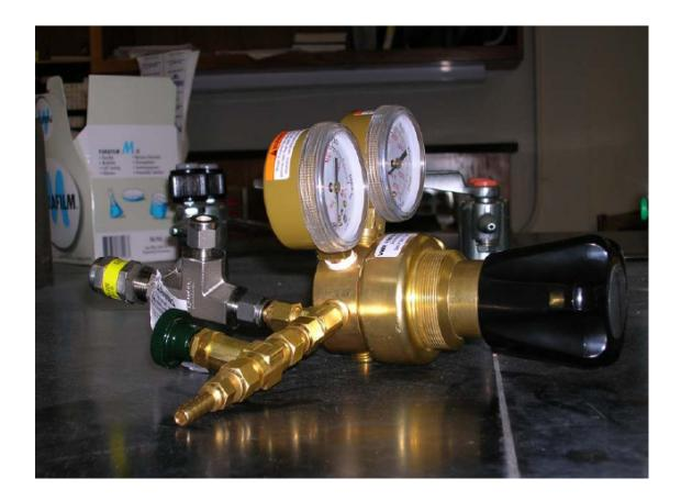
Then, adjust the safety valve to the pressure which is a little lower than the highest pressure the bottle can stand.
