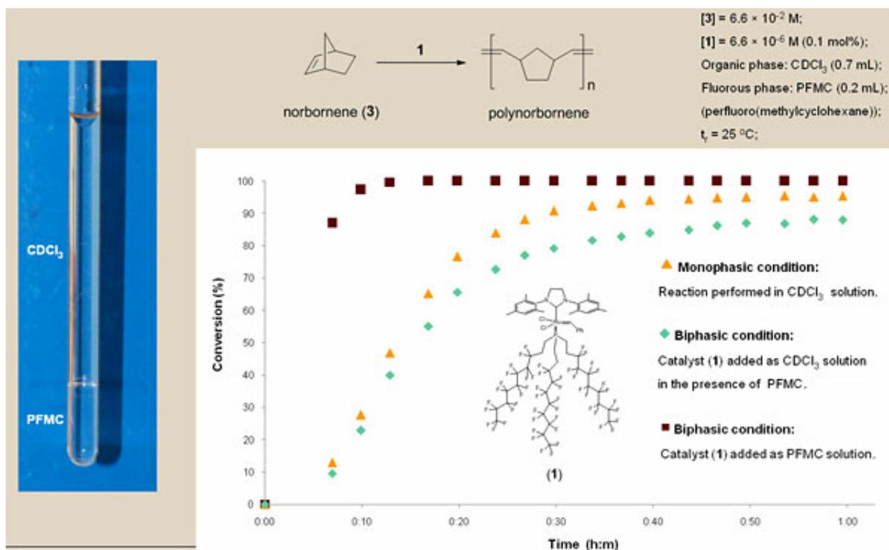
A liquid-liquid biphasic reaction system. (Image courtesy of Robert Tuba)
