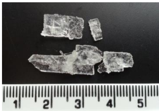
Figure S1. Representative single crystals of Ph 3 PO·(HO) 2 CMe 2 (4). The given scale is in cm units.
