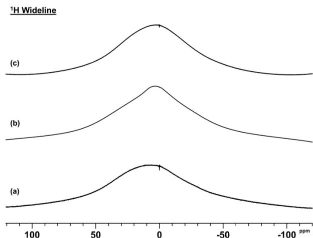
**Figure 9.** <sup>1</sup>H Wideline NMR spectra of the PEKK-PBI blend (a) as received, (b) after steam-treatment at 150 °C in H<sub>2</sub>O for 48 h, and (c) steam-treated at 150 °C in D<sub>2</sub>O for 48 h.
