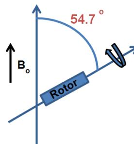
**Figure 1.** Principle of Solid-State Magic Angle Spinning (MAS) NMR.
