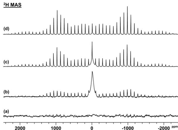
**Figure 8.** <sup>2</sup>H NMR spectra of PEKK-PBI (a) after treatment with D<sub>2</sub>O at RT, (b) after treatment with D<sub>2</sub>O at 150 °C, (c) immediately after being treated at 315 °C with D<sub>2</sub>O, and (d) 1 month after this treatment. The Pake Patterns with approximate quadrupolar coupling constants  $Q_{cc}$  of 160 kHz (b, c, d) are split into rotational sidebands (spinning frequency 6 kHz).
