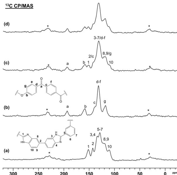
**Figure 3.**  $^{13}\text{C}$  CP/MAS NMR spectra of (a) PBI, (b) PEKK, (c) melt-blended PEKK-PBI, and (d) physical mixture of powdered PEKK and PBI (50:50 wt%). Rotational speed  $\nu_{\text{rot}} = 10$  kHz. The asterisks denote rotational sidebands.
