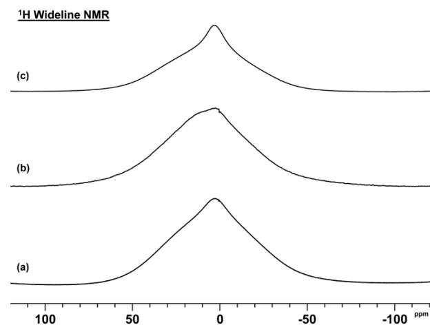
**Figure 10:** <sup>1</sup>H Wideline NMR spectra of the PEKK-PBI blend after (a) steam-treatment at 315 °C in H<sub>2</sub>O for 72 h, (b) steam-treatment of this sample at 315 °C in D<sub>2</sub>O for 72 h, and (c) after exposure to the atmosphere for 1 month.
