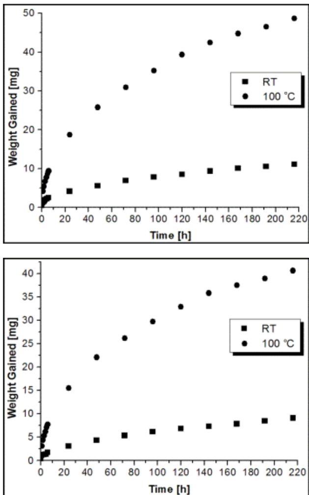
**Figure 6.** Weight gain of 1 g of PEEK-PBI (top) and 1 g of PEKK-PBI (bottom) when stirred in water at RT and at 100 °C.
