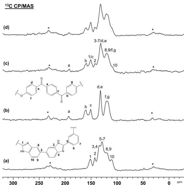
**Figure 2.**  $^{13}\text{C}$  CP/MAS NMR spectra of (a) PBI, (b) PEEK, (c) melt-blended PEEK-PBI, and (d) physical mixture of powdered PEEK and PBI (50:50 wt%). Rotational speed  $\nu_{\text{rot}} = 10$  kHz. The asterisks denote rotational sidebands.
