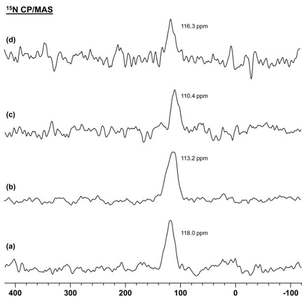
**Figure 4.** <sup>15</sup>N CP/MAS NMR spectra of (a) PBI steam-treated with D<sub>2</sub>O at 150 °C (6 kHz), (b) dried PBI (6 kHz), (c) melt-blended PEEK-PBI (10 kHz), and (d) melt-blended PEKK-PBI (10 kHz).
