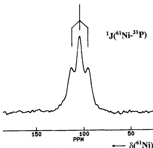
**Figure 2.** 26.8 MHz  $^{61}\text{Ni}$  NMR spectrum of  $(\text{CO})_2\text{Ni}(\text{PMe}_3)_2$ , dissolved in THF.  $^1J(^{61}\text{Ni}, ^{31}\text{P}) = 250 \pm 2$  Hz. Time required for the measurement: 3 h.
