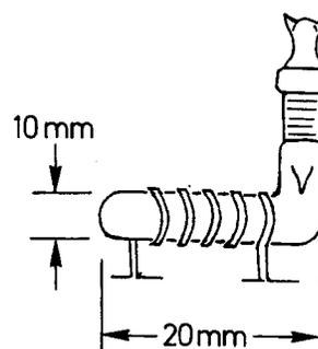
Figure 1. Schematic sideview of an airtight glass sample tube within the solenoidal coil of the probehead: The stopper (5 mm ground-glass joint) is fixed by a rubber band, which is not shown here. Diameter and length of the sample tube: 10 mm and 2 cm, respectively.
