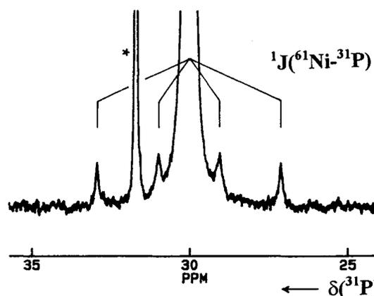
**Figure 4.** 121.5 MHz  $^{31}\text{P}$  NMR spectrum of a saturated THF solution of  $(\text{CO})_3\text{Ni}(\text{PPh}_3)_3$ . The asterisk denotes the  $^{31}\text{P}$  NMR signal of traces of  $(\text{CO})_2\text{Ni}(\text{PPh}_3)_2$ .
