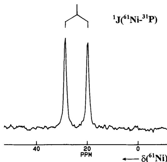
**Figure 3.** 26.8 MHz  $^{61}\text{Ni}$  NMR spectrum of  $(\text{CO})_3\text{Ni}(\text{PPh}_3)_3$ , dissolved in THF. Time required for the measurement: 0.5 h.
