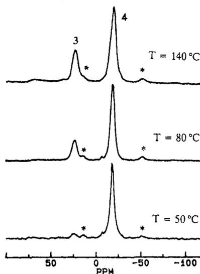
**Figure 4.** 121.5 MHz <sup>31</sup>P CP/MAS NMR spectrum of silica, modified with phosphine 1 at the given temperatures: 3 = side product; 4 = silica-immobilized phosphine 1. Asterisks denote rotational sidebands of signal 4.
