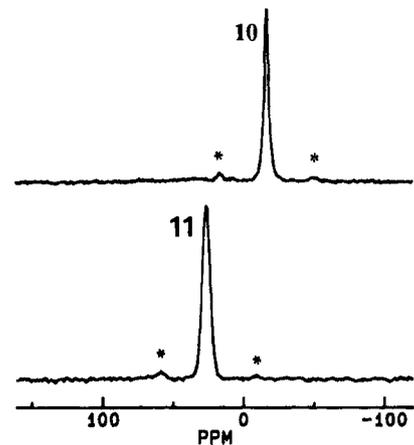
**Figure 7.** 121.5 MHz  $^{31}\text{P}$  CP/MAS NMR spectra of modified silica: top trace, immobilized (4-hydroxybutyl)diphenylphosphine (**10**); bottom trace, P(V) species **11**, prepared by treatment of **10** with  $\text{RSi}(\text{OEt})_3$ . Asterisks denote rotational sidebands.
