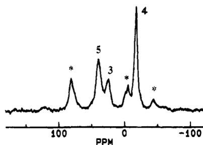
**Figure 2.** 121.5 MHz <sup>31</sup>P CP/MAS NMR spectrum of silica after immobilization of phosphine 1 in air: 3 = side product; 4 = immobilized phosphine; 5 = phosphine oxide. Asterisks denote rotational sidebands of signal 5.
