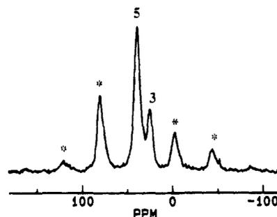
**Figure 3.** 121.5 MHz <sup>31</sup>P CP/MAS NMR spectrum of phosphine-modified silica 4, containing some side product 3, after oxidation with H<sub>2</sub>O<sub>2</sub>: 3 = side product; 5 = phosphine oxide. Asterisks denote rotational sidebands of signal 5.
