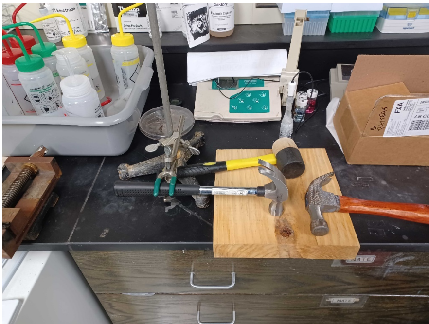
Figure 25. Hammers with wood, steel, and rubber faces along with a loosely controlled arm swinger for more repeatable motion.
