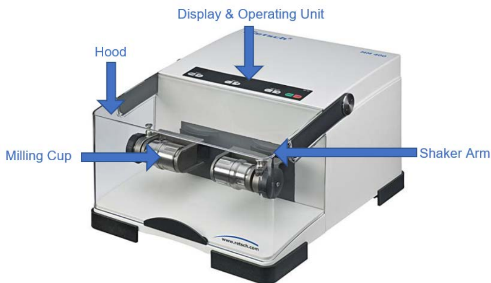
Figure 11. Retsch MM 400 ball mill used for performing mechanochemical reactions. Adapted from the Retsch MM 400 manual.
