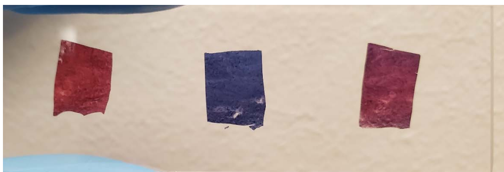
Figure 20. Mechanochromophore Films dipped into straight chain aliphatic hydrocarbons. The center film has not been exposed to solvent or mechanical force at all. The film on the left shows a greater progression towards red compared to the film on the right, allowing us to see that the inter-molecule bonds have been disrupted.
