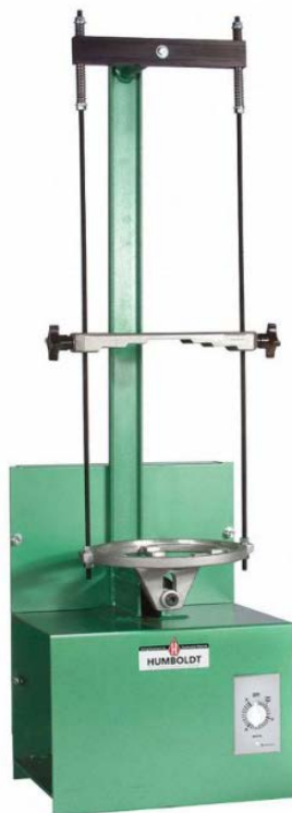
Figure 8. Humboldt sieve shaker adapted from https://www.grainger.com/product/HUMBOLDT-Hand-Operated-Sieve-Shaker-5DPL2 .
