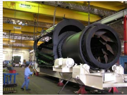
Hot mix plant being manufactured, Astec Industries
