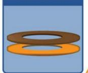
Valve Outlet Ensure free from dirt, PTFE tapes, oil and grease
