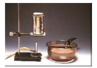
When can cools, vapor pressure of water drops. Pressure inside of the can is less than that of atmosphere, which collapses the can.
