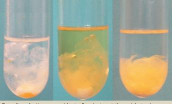
Recycling of a thermomorphic rhodium hydrosylation catalyst using *Teflon* tape
