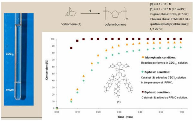
A liquid-liquid biphasic reaction system. (Image courtesy of Robert Tuba)
