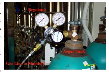
periodically. Do not exceed 15 psi pressure. Please notify the SDS manager(s) immediately if the tank is nearing empty (at or below 500 psi) or if a leak is suspected. Under normal operating conditions, an Argon tank should last for approximately 4-6 weeks.
