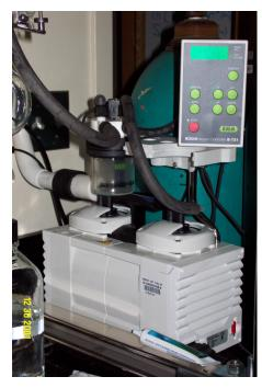
pump is turned on when the system is being used. The pump with the controller automatically turns the pump on and off to maintain a preset vacuum.
