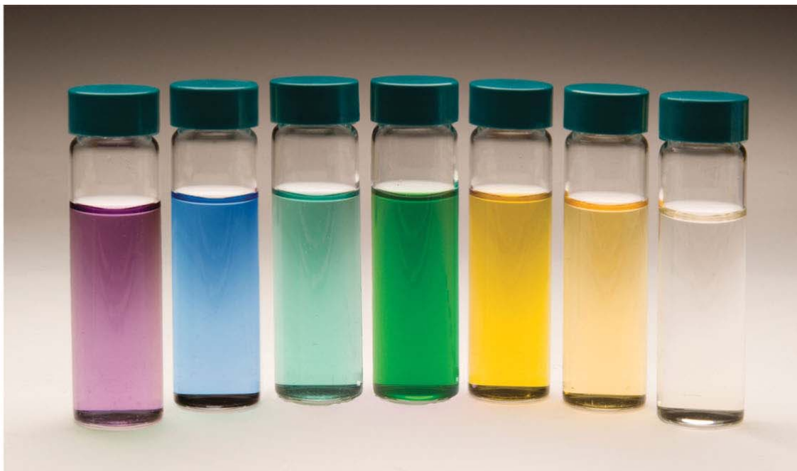
FIGURE 17.35 The effect on the color of the complex of substituting ligands with different ligand field strengths in octahedral cobalt(III) complexes in aqueous solution.
