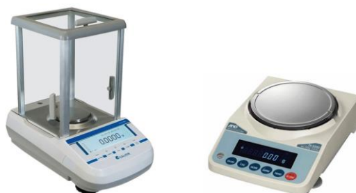
Figure 1. A digital Analytical Balance (left) and a digital Top loading balance (right).
