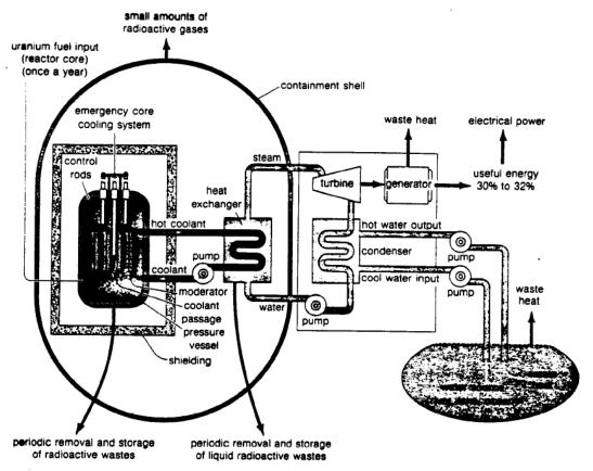
Figure 17.8 A nuclear power plant with a pressurized water reactor.
